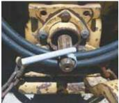
Edward Stanley, Parker, Texas: "Lining up my tractor pto is easy with my Porter pto alignment tool (porterprotools@aol.com; ph 972 742-0147). It comes with a 4 1/2-in. long pipe handle that has a sharply curved hook welded onto one end to grab a spline. I use this tool every time I hook up to a pto-driven implement. Sells for \$16.50 plus \$&H."
