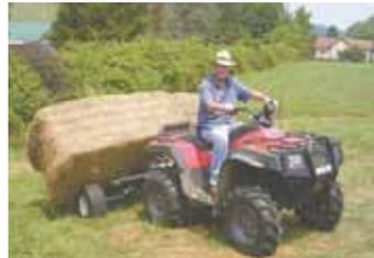
behind your 4-wheeler and can load and unload round bales weighing up to 1,200 lbs. with the push of a button (www.fasthaymovers.com; ph 304 282-1210). The unit attaches with a ball or receiver hitch and uses a bale spear, along with a small winch and pulleys, to lift and carry 4 by 4 and 4 by 5 bales.
