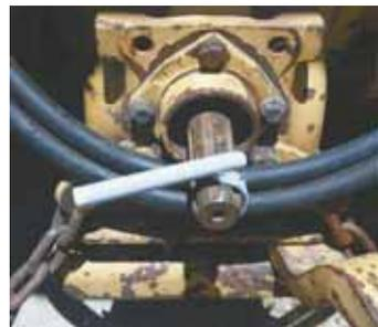
**Edward Stanley, Parker, Texas:** "Lining up my tractor pto is easy with my Porter pto alignment tool (porterprotools@aol.com; ph 972 742-0147). It comes with a 4 1/2-in. long pipe handle that has a sharply curved hook welded onto one end to grab a spline. I use this tool every time I hook up to a pto-driven implement. Sells for \$16.50 plus S&H."
