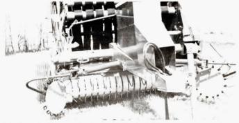
Tucker wheels extend effective pickup width 18 to 24 in. and can increase baler capacity 40 to 60%, says manufacturer.
