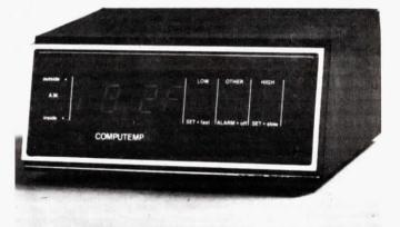
Computemp records the day's high and low temperatures and sounds an alarm when a preset temperature is reached.
