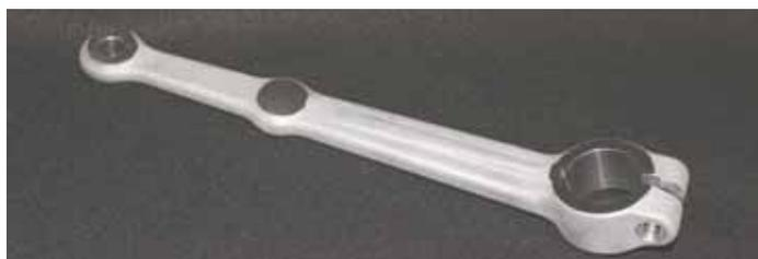
Eric Rego uses 3D machining to make replacement parts, such as the Oliver steering arm shown above.
