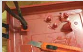
often sold in plastic tool cases mold-formed to contain a particular tool. Using a sharp utility knife, I convert such tool cases into handy, general purpose toolboxes that will never rust. The photo shows how I converted an 18-in. long, 14-in. wide, and 6-in. deep tool case to store a big hammer drill as well as drill bits and wall anchors.
