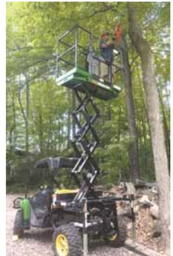
Battery-operated UTX scissor lift turns a side-by-side utility vehicle into a mobile lift station.
