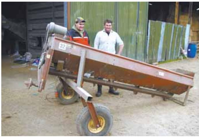
David Treharnes in England built his own low-cost, portable grain cleaner by mounting 2 custom-built augers inside an old grain drill box.
