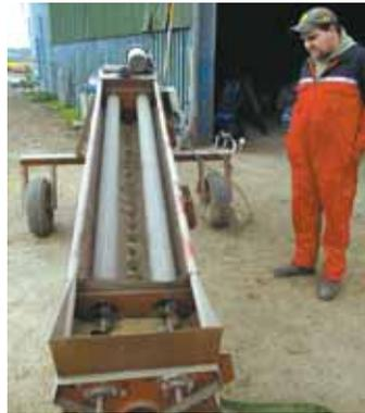
Grain is pulled by augers through perforated metal tubes, allowing waste material to drop through onto the ground.
