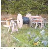
Electric cable spool mounts on a metal pole that rests on 2 sawhorses.
