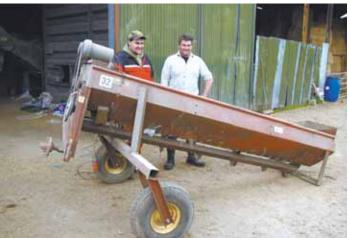
David Treharnes in England built his own low-cost, portable grain cleaner by mounting 2 custom-built augers inside an old grain drill box.
