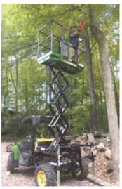
Battery-operated UTX scissor lift turns a side-by-side utility vehicle into a mobile lift station.
