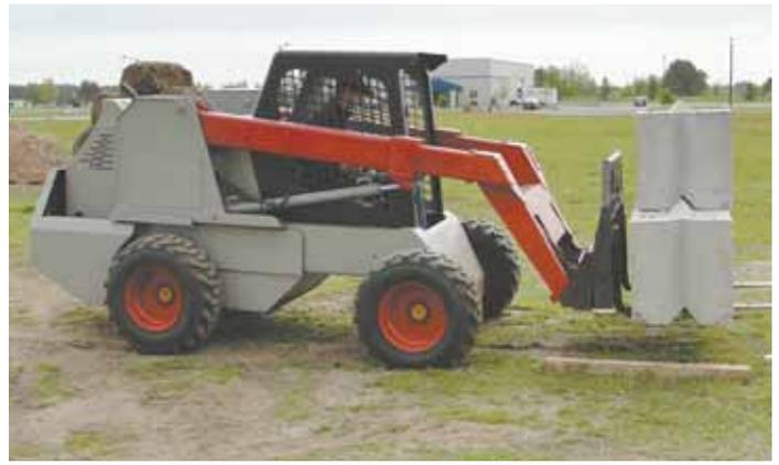
New skid loader has telescoping loader arms and an extendable wheelbase that lengthens out to 84 in., allowing it to lift heavier loads.
