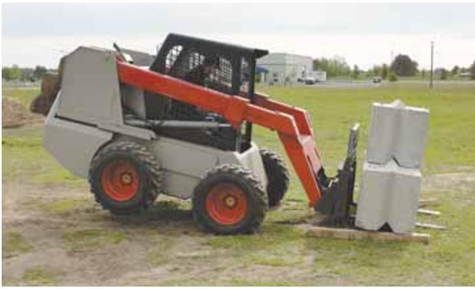
Pro-Handler skid loader can lift a 5,000-lb. payload 14 ft. in the air. "It'll outperform the biggest skid steers on the market," says the company.
