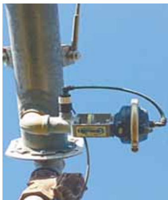
EndFlush automatic flushing device cleans center pivot irrigation pipes at the beginning and end of each watering cycle.
