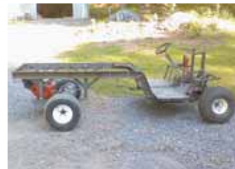
Power is supplied by a 16 hp Honda-clone engine mounted on back of truck frame.
