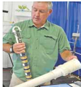
Electronic sensors on probe detect plant response across various soil types, moisture, and fertility levels, at various stages of plant growth.
