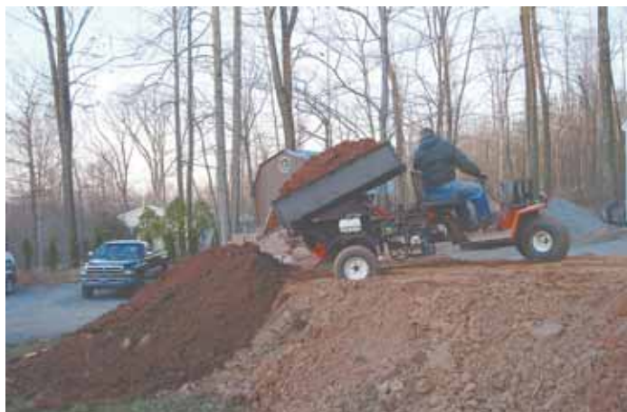
Andrew Salisbury's home-built mini dump truck is sized to handle several scoops from his compact Kubota loader tractor.
