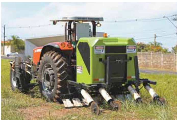
A Brazilian company that makes machines designed to kill weeds with electricity, plans to sell and lease equipment in North America.
