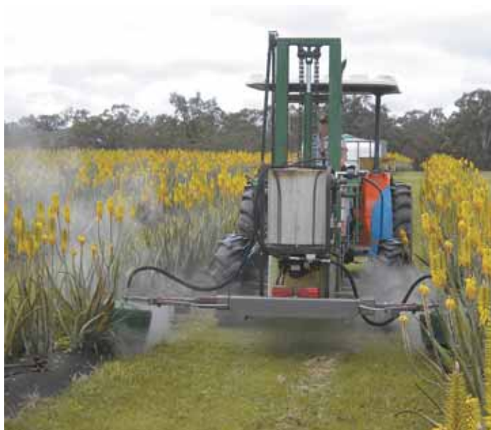
An Australian company has developed saturated steam generators that kill weeds in a single pass. Several machines are available including this one that supports 2 applicator heads.
