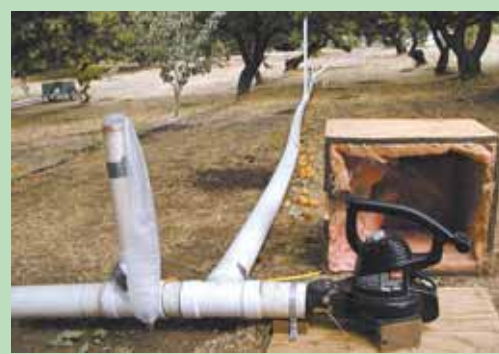
Electric leaf blower, housed under insulated wood box to reduce noise, is plumbed to a pvc pipeline with a series of vertical outlet pipes fitted with tube-shaped plastic bags. When blower starts up, the plastic tubes expand and flap around, scaring birds.
