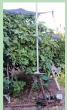
Another type of scarer is a rotating mast with a cross arm on top dangling milk jugs, plastic streamers, and a variety of other items. A gear-reduced shaft drives the mast.
