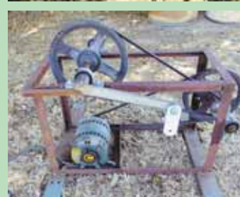
The “rope-a-dope” scarer, above, consists of several light ropes strung through multiple trees. An offset crank arm, left, tugs and releases ropes, shaking items dangling from them to scare birds.
