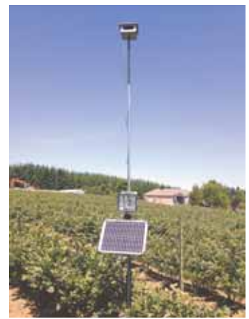
Bird Gard audio system uses randomized patterns of distress calls to scare away pest birds permanently.
