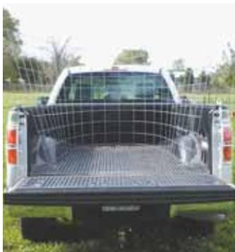
U-shaped panel is placed on pickup bed (left). After animal is in pickup, the 2 loose panel ends are pulled together. Cage is then tied to stake hole inserts.
