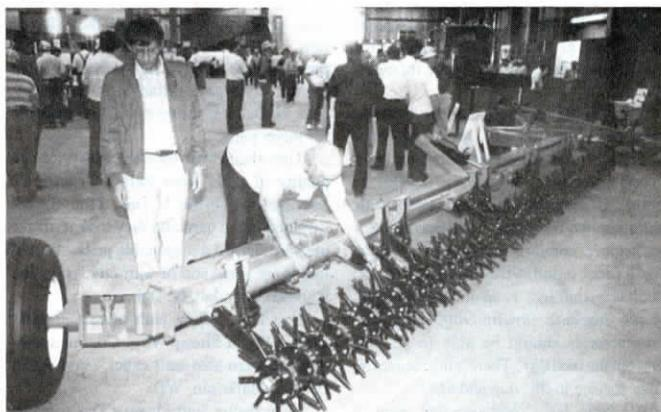
**Harrow consists of a series of discs, each supporting eight 6-in. long steel spikes.**
