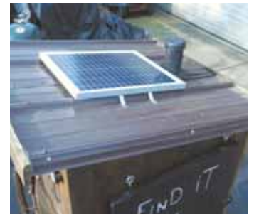
Sensor probes in the smoker are wired to a controller, which in turn runs a small compressor that delivers air to smoker's charcoal bed. A solar panel on roof powers the controller.
