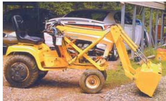
"It's fun to operate and easy to handle," says Carman Fedele about the front-end loader he built for his Cub Cadet 1440 garden tractor.
