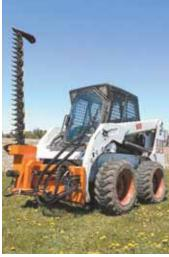
Mower folds up vertically for transport and downward for roadside clearing.
