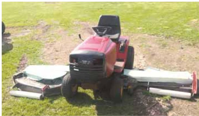
Murray 42-in. riding mower is flanked by matching side decks, which overlap the middle deck by 3 in. and can flex up and down.
