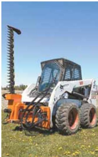
Mower folds up vertically for transport and downward for roadside clearing.
