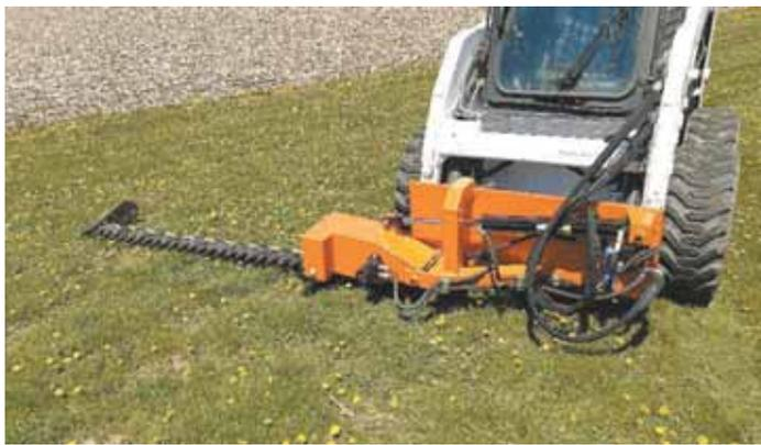
"It's handy for doing a variety of farm work," says Andrew Lee, who converted a New Idea pto-powered, 7-ft. sicklebar mower to hydraulic-drive for use on his Bobcat skid loader.
