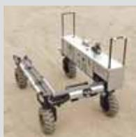
Powered "platform" has 4 hydrostatically-driven wheels.
