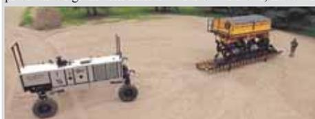
Grain drill (right) was designed to fit platform, which drives under and lifts it into place before heading to the field.
