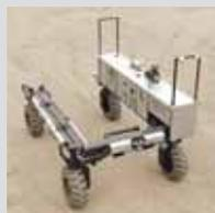
Powered "platform" has 4 hydrostatically-driven wheels.
