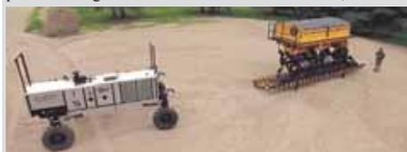
Grain drill (right) was designed to fit platform, which drives under and lifts it into place before heading to the field.
