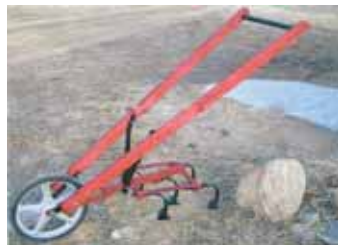
Cultivator has 3 rows of staggered shanks with 3 1/4-in. wide shovels welded onto them. The design leaves no gap. Shovels have hocks on back to pull weeds, if needed.
