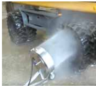
Hurricane Pro undercarriage cleaner blasts streams of water out of rotating nozzles on a 3-wheeled cart. Spray deck can be pivoted from flat to 90 degrees vertical.
