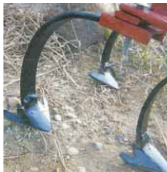
Cultivator has 3 rows of staggered shanks with 3 1/4-in. wide shovels welded onto them. The design leaves no gap. Shovels have hocks on back to pull weeds, if needed.
