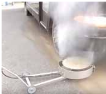
Hurricane Pro undercarriage cleaner blasts streams of water out of rotating nozzles on a 3-wheeled cart. Spray deck can be pivoted from flat to 90 degrees vertical.
