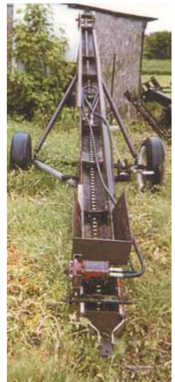
Roger Reibsamen used a pair of combine return elevators to make this low-cost elevator. He uses it to load firewood into a woodshed.
