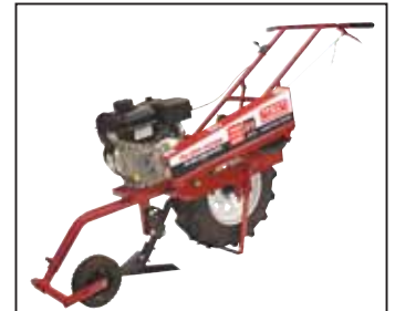
One-wheeled Plow Boss is powered by a 127cc Briggs & Stratton engine. It comes with interchangeable accessories including a turn shovel, 12-in. sweep, and furrower.
