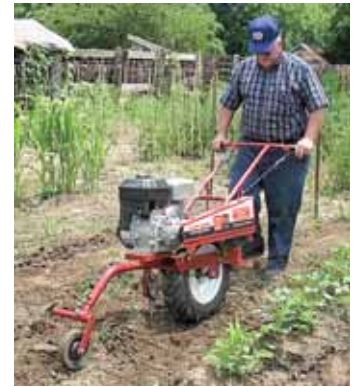
One-wheeled Plow Boss is powered by a 127cc Briggs & Stratton engine. It comes with interchangeable accessories including a turn shovel, 12-in. sweep, and furrower.
