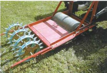
Clark designed and built this "packer-dibbler", which is used to make holes in the ground for transplanting bulbs and seedlings.
