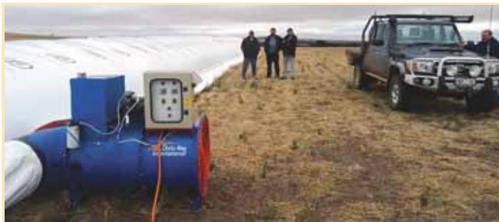
Grain is loaded into bag with standard bagging machine. Dryer hooks to plastic tube on side of bag, sending warm air through grain and out tube on other side of bag.
