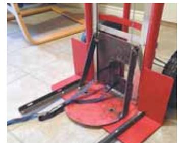
Two pieces of angle iron on base keep 2-wheeler from tipping forward when lifting a load.
