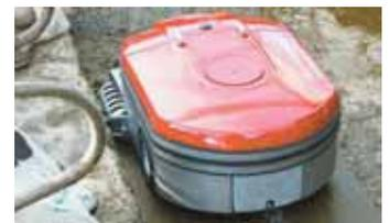
**Lely manure robot is designed to vacuum up manure in dairy barns. Cows just step around it as it makes its rounds.**
