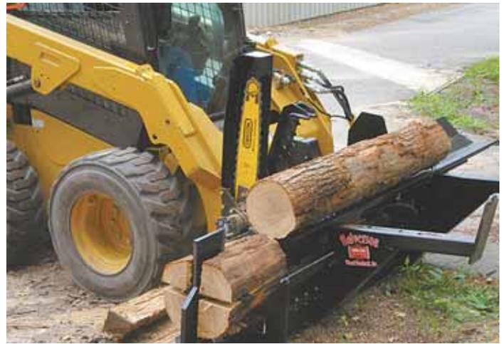
**One-man firewood processor is a combination log fork, squeeze arm, chainsaw and log splitter. It attaches to skid loaders with a universal mount.**
