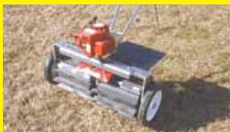
I recently developed a wheel kit and power sweeper attachment for Mantis rototillers. I adapted another vendor's sweeper drums to the rototiller and also incorporated a wheel kit, which makes
