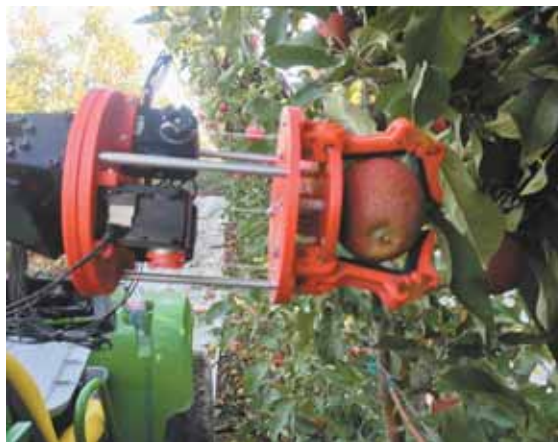
Karkee robotic apple picker uses pressure sensitive "hands" to harvest fruit without bruising, breaking or puncturing it.
