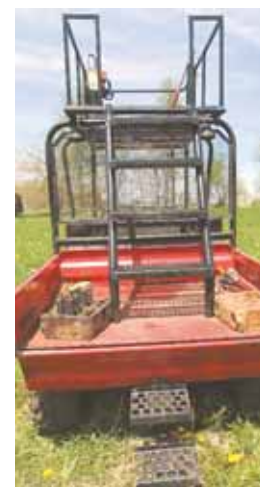
Working platform is 6 ft. off the ground. Pivoting T-brackets fit over front bumper (left). Two heavy cylinder heads in back help anchor the rear end (above).
