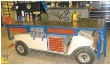
Montezuma toolbox mounts on one side of workbench behind driver, and there's a fold-out compartment covered by an expanded metal "rack" on front for tool storage.
