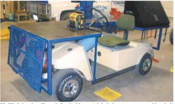
Modified electric golf cart is fitted with a metal deck that serves as a workbench. It wraps around 3 sides of vehicle and attaches to it with 4 bolts on front and back.
