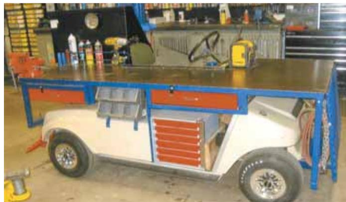
Montezuma toolbox mounts on one side of workbench behind driver, and there's a fold-out compartment covered by an expanded metal "rack" on front for tool storage.
