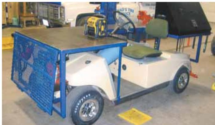
Modified electric golf cart is fitted with a metal deck that serves as a workbench. It wraps around 3 sides of vehicle and attaches to it with 4 bolts on front and back.
