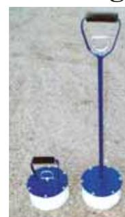
“Quick release” magnet comes with a 5-in. dia. magnet contained in a pvc housing with an aluminum base. When you pull trigger, magnet pulls away from base and the object drops off.
