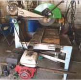
at an auction for \$20 and converted it to a portable steel-cutting chopsaw. The saw's electric motor didn't work so I replaced it with a Honda 9 hp gas engine. I also installed a new driveshaft and replaced the saw's belts and pulleys to fit.
