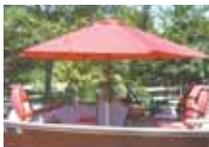
**Umbrella mounts on boat's side-steer console with a pvc pipe and 2 straps. Clevis pin provides 3 height options.**
