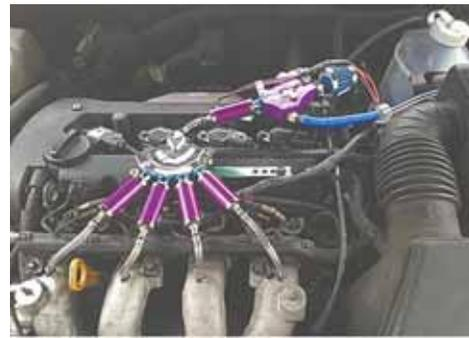
Aquatune fuel system injects hydrogen directly into engine ahead of combustion, improving conventional fuel combustion.
