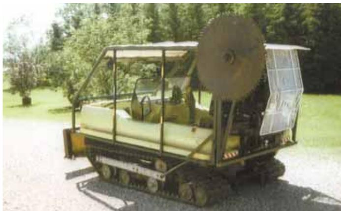
Big 32-in. dia. sawmill blade mounts 6 ft. off the ground alongside ATV's rollbar. As Nielsen drives along, bent-over small trees are cut by blade.
