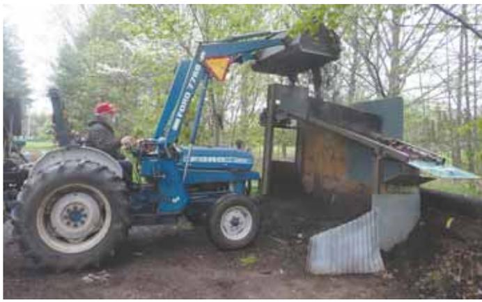
Rod Stremlo's big home-built sifter is able to handle compost using a front-end loader. There's room underneath for loader to retrieve a bucketful of sifted compost.
