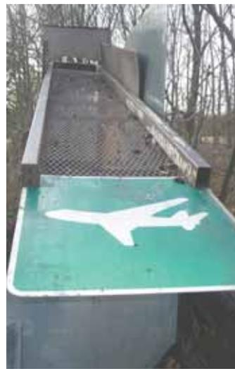
The 2-ft. wide by 12-ft. long sifter mounts on a frame made from old goal posts and steel tubing.
