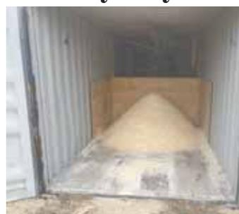
Ground corn is dumped onto a pile for removal by skid steer.
