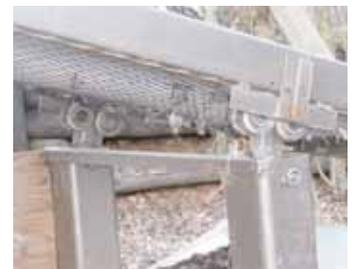
Screen frame rides on plastic wheels mounted to uprights on main frame. Offset drive with springs provides screen with 1 1/2 in. of lateral movement with each revolution.
