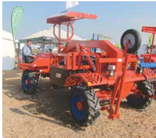
Designed mainly for vegetable crops, Scorpion self-propelled automatic weeder can remove weeds between the rows and also between plants in the row.
