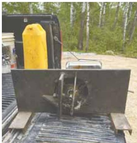
Jig consists of a 1/2-in. thick steel plate welded at a 90-degree angle to a larger plate that’s big enough to bolt engine in place. Mower shaft protrudes through hole cut into center of plate.
