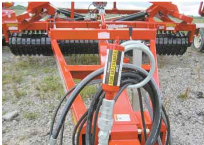
When inactive hoses are coupled to the Hose End Chamber, it relieves hydraulic pressure buildup in the hoses.
