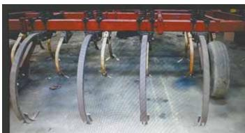
"Track Tillage" implement has 9 chisel plow shanks on back and 2 rows of field cultivator shanks on front that line up exactly with those on back. Shanks dig progressively deeper from front to back.
