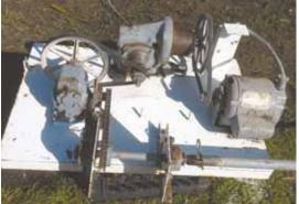
With the help of 2 gear reduction motors and 6 sprockets, Richard Berry built this whole hog rotisserie. It turns hog just once every 4 1/2 min.
