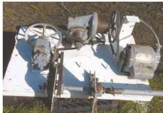
With the help of 2 gear reduction motors and 6 sprockets, Richard Berry built this whole hog rotisserie. It turns hog just once every 4 1/2 min.
