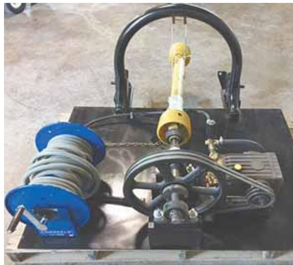
Jake Iftner's 3-pt. mounted, pto-powered pressure washer is made mostly from off-the-shelf components except for the power transfer shaft, which was fabricated at a local machine shop.
