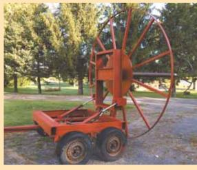
Home-built, tandem axle tile trailer is designed to hold a roll of drainage tile vertically for transport, then tip it back in the field to unroll.
