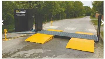
Spraying starts automatically when vehicle drives over ramp. Disinfectant is sprayed through nozzles in the floor and 2-ft. tall side screens and reaches all around the wheels.
