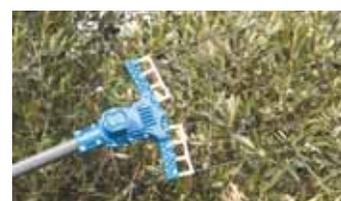
Powered by a 12-volt battery, rake head uses 8 carbon fiber teeth to shake the branches, detaching olives.
