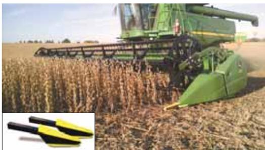
ExoPlate Crop Dividers are shorter than the crop divider snouts on many grain heads, and knock down fewer soybeans when making sharp turns or adjusting to auto track.
