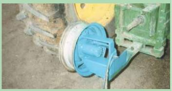
Wire roller pins onto tractor drawbar and plugs into tractor's hydraulic outlets. It's operated by the hydraulic motor off an old swather reel.
