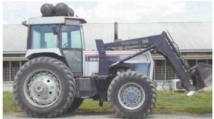
Danny Kluthe came up with a way to compress and purify biogas from manure to use as a diesel fuel alternative. He runs his White diesel tractor on 90 percent compressed methane and 10 percent diesel (above). He and partner Kevin Kenney are now marketing the system.
