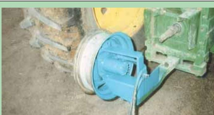
**Wire roller pins onto tractor drawbar and plugs into tractor's hydraulic outlets. It's operated by the hydraulic motor off an old swather reel.**
