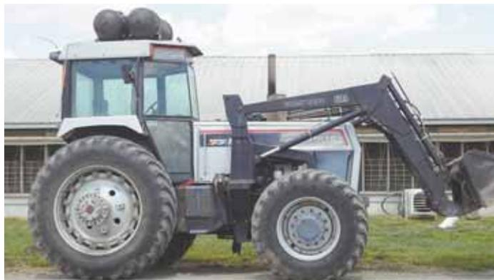
**Danny Kluthe came up with a way to compress and purify biogas from manure to use as a diesel fuel alternative. He runs his White diesel tractor on 90 percent compressed methane and 10 percent diesel (above). He and partner Kevin Kenney are now marketing the system.**
