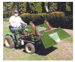
Dennis Gintowt built this front-end loader for his 1972 Deere 112 garden tractor. With weights on back of tractor he can pick up as much as 500 lbs. Hydraulic pump is belt-driven off the engine and positioned so it doesn't hit tractor's front wheel.
