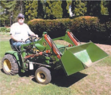
Dennis Gintowt built this front-end loader for his 1972 Deere 112 garden tractor. With weights on back of tractor he can pick up as much as 500 lbs. Hydraulic pump is belt-driven off the engine and positioned so it doesn't hit tractor's front wheel.
