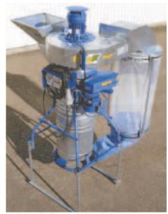
Polish-built Sosnowski seed cleaner uses centrifugal force to remove trash from all types of seed.
