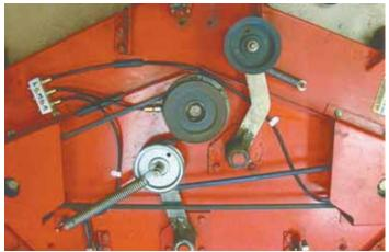
Home-built manifold block distributes grease through individual lines to each grease point on Glander's mower deck.
