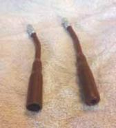
Grease gun extension lets you apply down pressure on a zerk that would otherwise allow grease to squirt out the side.
